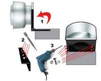
4. (A) After hinges are mounted to the fan base and fan duct, carefully tilt the fan back so to have access to the bottom of the fan base. (B) Using a punch, mark through the pre-drilled holes on top of angled mounting brackets so accurate drilling holes for the supplied upper mounting bolts can be made. (C) Drill the holes using a 1/4" drill bit. Fasten bolts through brackets and fan base. Be sure to install the washers before fastening the bolts.
